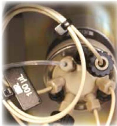
Exchangeable Sample Loop made of PEEK
