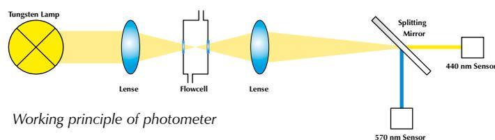
Working principle of photometer
