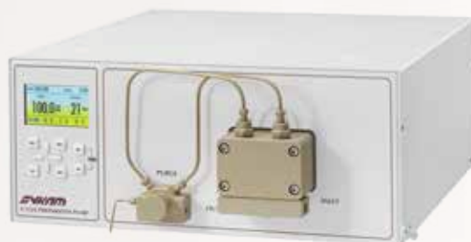
The S 1525 Preparative Pump, with metal-free PEEK pump heads, a flow rate range of up to 1000 ml/min and pressure range of up to 350 bar
