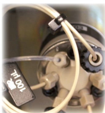
Exchangeable Sample Loop made of PEEK
