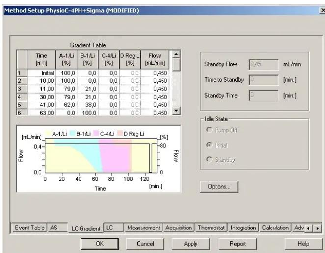
All method parameters are stored within the chromatogram datafile. Buffer gradient, column temperature gradient, integration and calculation parameters as well as the actual buffer- and reagent pressure and actual column temperature are recorded during the run. The buffer gradient program is shown here as one of the tabs of the method screen.
