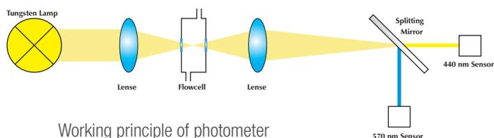
Working principle of photometer
