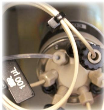
Exchangeable Sample Loop made of PEEK
